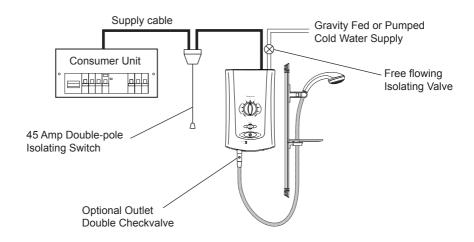
**Electrical Schematic Diagram**
