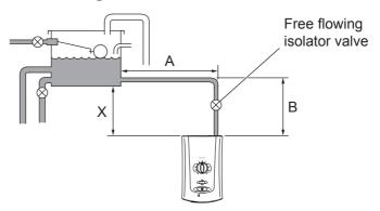
**Example!** The example below is based on the diagram above with 15 mm pipework, A = 1.5 m, B = 0.75 m.
