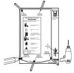
Use template provided to mark and drill required fixing holes. Screws and plugs are supplied for 4 holes.
