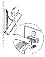
**15.** Connect ribbon cable to the inside of the cover.
