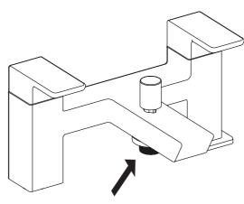
To change the original direction of the hose connection, loosen the screw found on the diverter, change the direction and tighten the screw.
