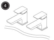
Connect the hot and cold water supplies to the threaded tails using either a ½" or ¾" BSP connector (not supplied).
