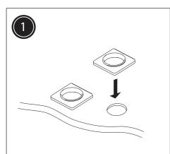
Place the plinths over the holes in the basin ensuring that the washers are fitted between the plinths and the basin/bath.
