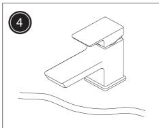
Connect the flexi/ copper tails to the hot and cold water supplies. Turn on the mains water supply letting the water flow for a few minutes to flush through the system. Check all joints and connections for any leaks.
