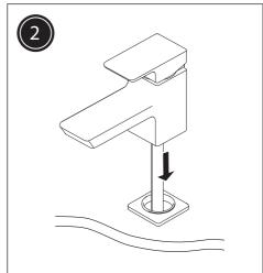
Place the plinth over the hole in the basin/ bath and feed the flexi tails through.
