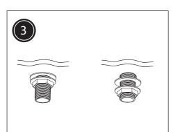
Secure the tap bodies to the basin/bath by using the washer and metal backnut below the basin /bath. Tighten the backnut onto the threaded tails. A suitable spanner may be required to fully tighten the backnut.
