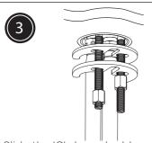
Slide the 'C' shaped rubber washer and the 'C' shaped metal washer onto the fixing rods up to the underside of the basin/ bath. To secure the tap body in place tighten the fixing nuts onto the fixing rods until they fully tightened against the 'C' shaped metal washer. A suitable spanner can be used to fully tighten the fixing nuts.
