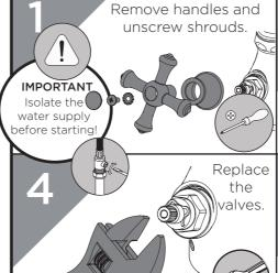
Remove the valves using a suitable spanner.
