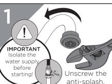
Remove the anti-splash and filter from housing. Clean and replace as necessary.
