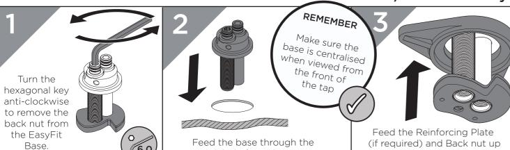
Feed the base through the sink hole from the top.
