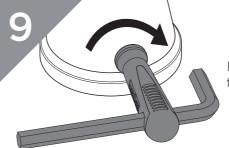
hexagonal key through the EasyFit tool and tighten the grub screws with an extra 1/2 turn.
