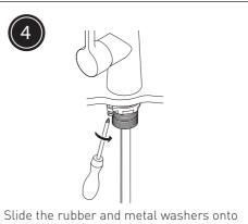
Slide the rubber and metal washers onto the thread and secure in place by tightening the backnut up to the underside of the basin. The screws on the backnut allow for any uneven surfaces and should be tightened up to the metal washer.
