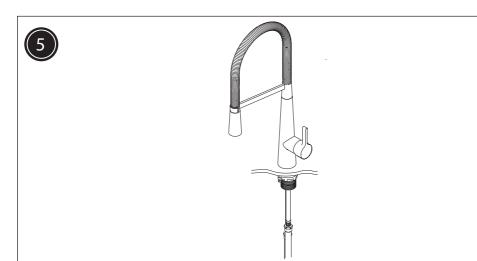
Connect the flexi tails to the hot and cold water supplies. Turn on the mains water supply letting the water flow for a minute to flush through the system. Check all joints and connections for any leaks.
