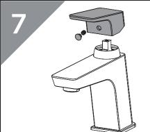
Replace the handle, tighten the grub screw and push fit the cap
