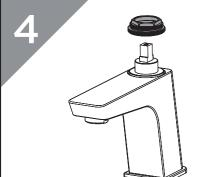
Remove the cartridge retaining nut using suitable spanner.
