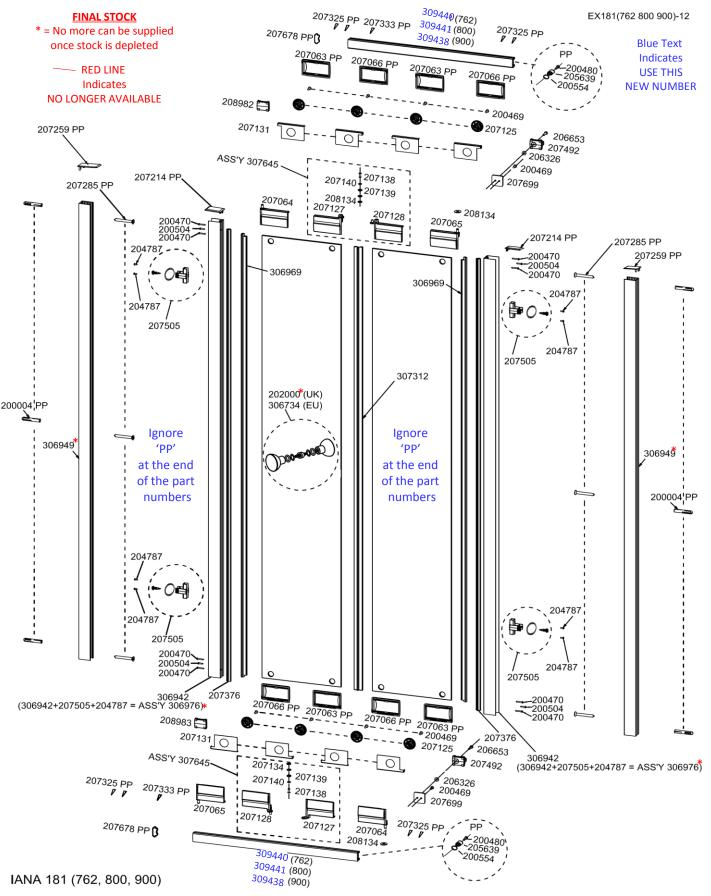
To ensure correct replacement parts are sent be ready to quote the six digit code from this drawing e.g. 304781
