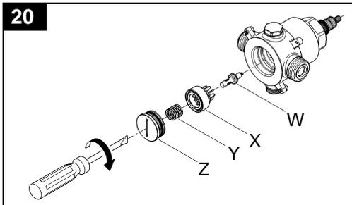
5. Tighten seat (Z) in the valve body.
