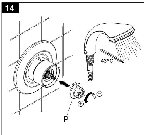
3. Check the temperature of the outflowing water with a thermometer.
