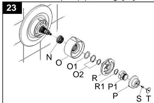
17. Push on shut-off handle (O) in closed position.
