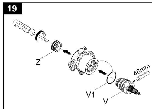
2. Reinstall O-ring seal (V1).
