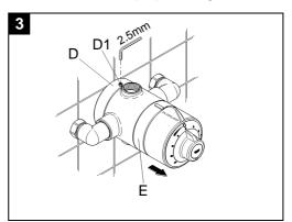
5. Remove valve body (E) from supply pipes and hold backplate (D) in position.
