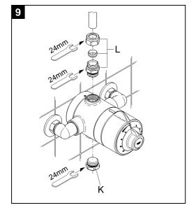
2. Thread the outlet nipple (L) with the O-ring seal into the valve body outlet.
