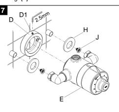
Slide the valve body (E) with elbows and compression nuts loosely over the supply pipes.
