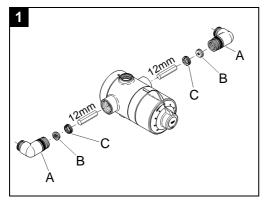
• Install flow limiters (B) in accordance to table above with threaded rings (C) by using a 12mm socket spanner.
