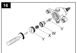
5. Close control unit (U) by turning the unit stem clockwise to closed position.6. Tighten seat (Y) in the valve body.
