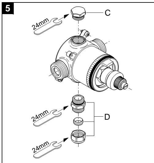
3. Thread the outlet nipple (D) with the O-ring seal into the valve body outlet.
