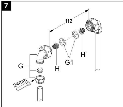
2. Install filters (H) and seals (G1) into the elbows (H).
