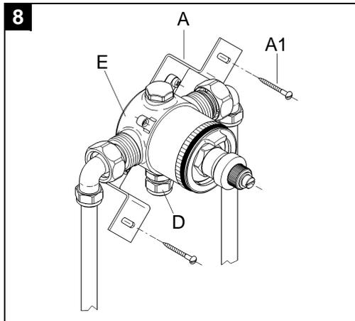
4. Connect mixed water supply to the outlet nipple (D).
