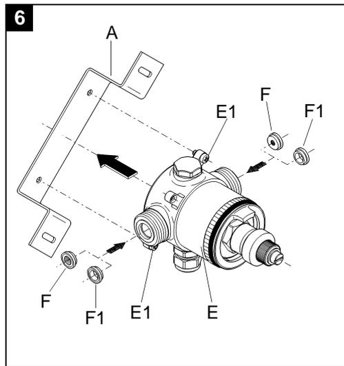
5. If there is a pressure differences between the hot and cold water supply install attached flow limiters (F) or spacers (F1) in the hot and cold water connection inlets, see table below.
