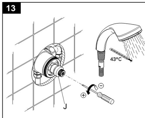
6. With a small screw driver adjust temperature to 43 °C. Turn clockwise (to reduce temperature) or counter-clockwise (to increase temperature).
