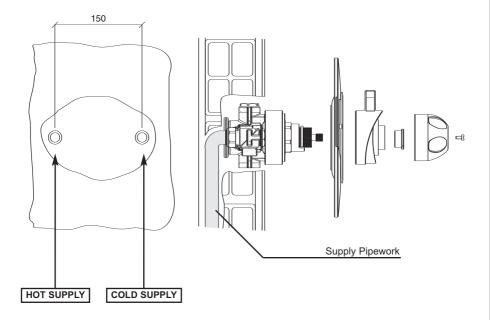
Optional wall elbow available on request for concealed installation with flexible hose kits.
