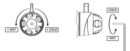
Turn the temperature control back to the maximum hot setting and measure the outlet temperature, when stabilised with a calibrated thermometer.
