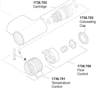
1736.707 Screw Pack - Components Identified 'A' 1736.708 Seal Pack - Components Identified 'B' 1736.717 Component Pack - Components Identified 'C'
