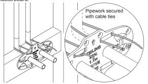
Important! Failure to secure the pipework may result in the pipework pushing back into the wall when fitting the mixer valve.
