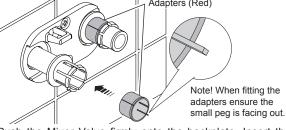
14. Push the Mixer Valve firmly onto the backplate. Insert the retaining screw into the Mixer Valve and tighten with the 2.5 mm hexagonal key (supplied).
