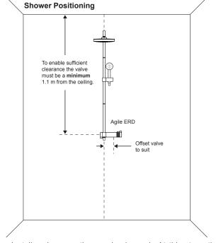
Install and secure the supply pipework. At this stage the pipework should extend a minimum of 50 mm from the finished
