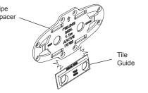
Important! The mixer valve will not be level If the supply pipe stubs exiting the wall are not level, use a spirit level on the flat surface of the pipe spacer to confirm that it is level before securing the spacer to the noggin.
