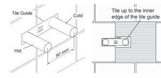
Using a pipe slice, trim the protruding pipework to 24 - 29 mm. **DO NOT** use a hacksaw as the sharp edges may damage the seals in the mixer valve. Note! De-burr the pipework if necessary.
