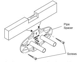
Screw the pipe spacer to the noggin, using a minimum of 2 screws. If the pipework is not rigidly secured use the cable ties supplied. Ensure it will not interfere with the finished plasterboard
