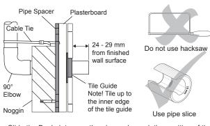
10. Slide the Backplate over the pipework, mark the position of the screw holes. Note! Ensure the backplate is fitted the correct way, with the hook to the left.
