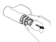
Grip the stop assembly and withdraw the cartridge from the body.
