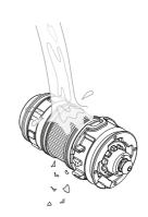
Rinse the cartridge in clean warm water, removing any dirt or debris.
