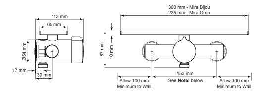
Note! If you are retro-fitting your mixing valve onto existing pipework, an Adjustable Elbow Pack is available if required, refer to section: 'Accessories'.
