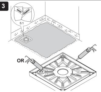
Install the shower tray on a bed of sand and cement or silicone sealant.
