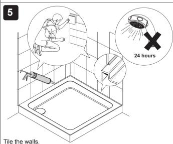
Apply silicone sealant in accordance with the manufacturer's tions to seal the shower tray to the tiled wall surface
