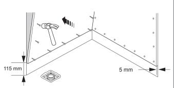
Apply silicone sealant in accordance with the manufacturer's
