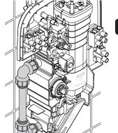
pipe to the inlet connector using a push fit elbow or an elbow with compression nuts and olives. Turn on the water supply
