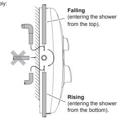
Note! - DO NOT use an incoming supply entering the shower directly from the back. Add an elbow to the supply pipe and connect it as a rising or falling supply.
