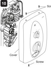
Ensure the control dials are aligned with the spindles and replace the cover.
