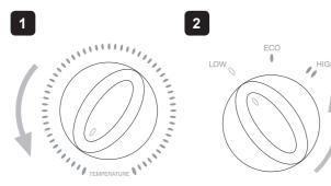
Turn temperature control to the Turn power control to low. cold position.
