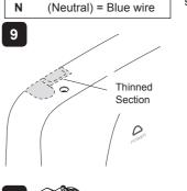
For falling or rising supplies the cover has thinned sections on the top and bottom that can be removed to allow entry of the supply pipe and electrical
