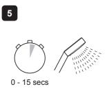
Water flows freely within a few Turn power control to Eco. seconds, temperature remains cool
