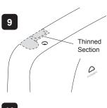
For falling or rising supplies the cover has thinned sections on the top and bottom that can be removed to allow entry of the supply pipe and electrical cables
