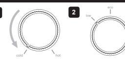
Turn temperature control to the Turn power control to low. cold position.
