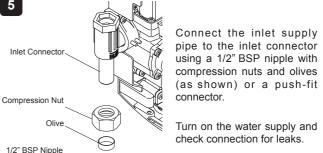
Connect the inlet supply pipe to the inlet connector using a 1/2" BSP nipple with compression nuts and olives (as shown) or a push-fit
