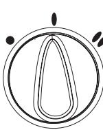
9. Turn the **TOP** knob to the **HIGH** position. The temperature of the water will rise further - this shows that the full power setting is operating correctly.
