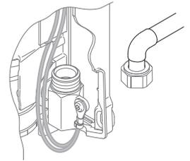
4. Remove front cover. Determine supply pipe position.
