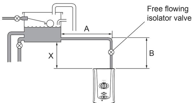
**Example!** The example below is based on the diagram above with 15 mm pipework, A = 1.5 m, B = 0.75 m.
