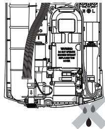
**10.** Drill holes through plastic case as required. Fix appliance to wall. (Make sure rubber feet are fitted with all holes used.)
