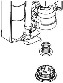
3. Unscrew the filter cap. Remove, clean and refit, or replace the filter as necessary. Refit the filter and the filter cap, making sure it is screwed fully home.
