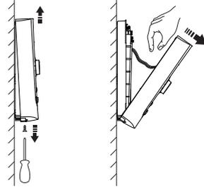
2. Remove the cover screw, cover and splash guard. Disconnect the ribbon cable from the cover
