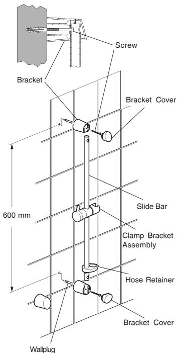
**1.3.** For solid walls drill two 8.0 mm diameter holes at 600 mm centres and insert the wall plugs.
