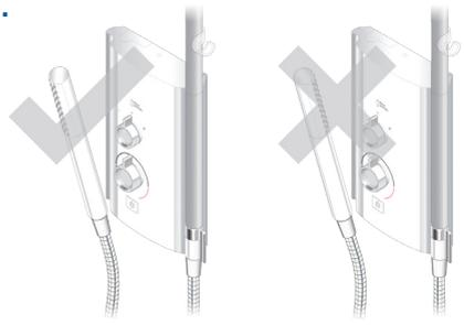
When storing handset, make sure spray nozzles are always pointing away from main unit.
