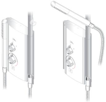
Handset may be kept on handset holder or magnetically attached to main unit (Part A).
