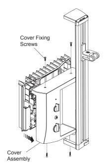
5. Remove the four screws that attach the cover assembly.
