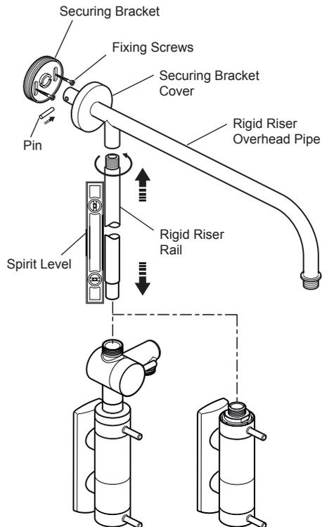
20. For **ER** models slide the concealing plate, compression nut and olive onto the rigid riser rail and locate it into the mixer outlet.
