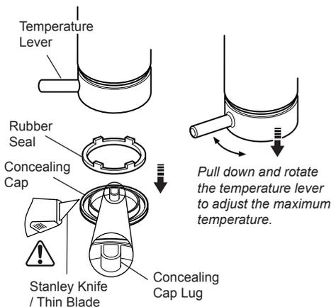
6. Once the maximum temperature is satisfactory, tighten the securing screw.
