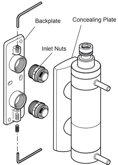
6. Using the backplate as a guide, mark the positions of the fixing holes and the pipe centres.
