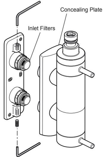
13. Push the concealing plate onto the backplate, secure with the M4 x 12 mm grubscrew.
