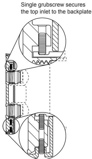
Two grubscrews secure both the bottom inlet and the concealing plate to the backplate
