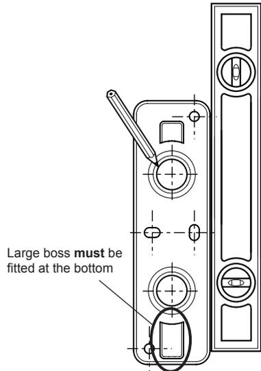
7. For solid walls drill the fixing holes for the backplate with a 6 mm drill and insert the wall plugs (supplied). For other types of wall structure alternative fixings may be required (not supplied).
