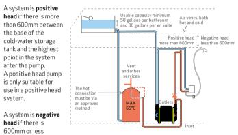
between the base of the cold-water storage tank and the highest point in the system after the pump. You can check if you have a negative head system by timing how long it takes to fill a measuring jug. You have a negative head system if:
