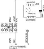
Fig. 7 230 VAC/1PH/50Hz SUPPLY 3.20 **Fuse:** All models should use 5 Amp fuse.
