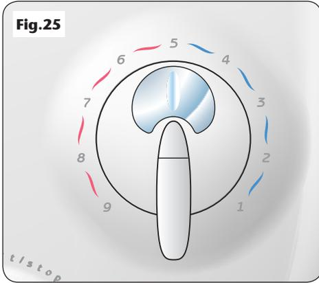
onto the splined spindle. When fitting the temperature control, the pointer must relate to the '5' on the temperature scale when the cover is fitted (**fig.25**). Refit the retaining screw and push fit the cover trim back into place.
