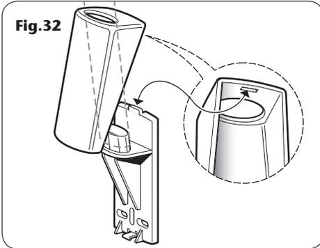
To remove a trim, push a small screwdriver or similar through the slot in the trim end and carefully pull away from the wall bracket.
