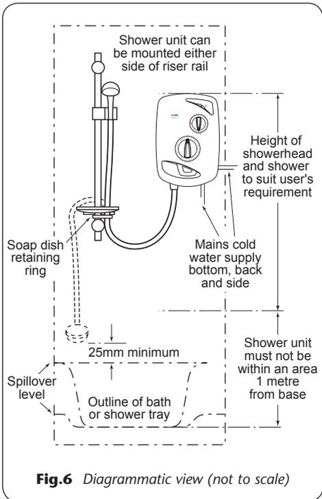
**Fig.6** Diagrammatic view (not to scale)
