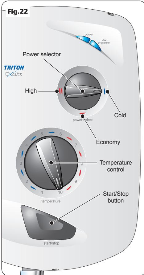
**Note:** In normal use, it is in order to leave the water supply permanently on to the shower unit, but as with most electrical appliances, **the unit must be switched off at the isolating switch when not in use.**
