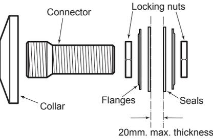
The maximum thickness of wall is about 20 mm. Enough room must be left on the connector to fit the compression nut and olive. At the front end, an allowance **MUST** be made to accept the shower union and collar.
