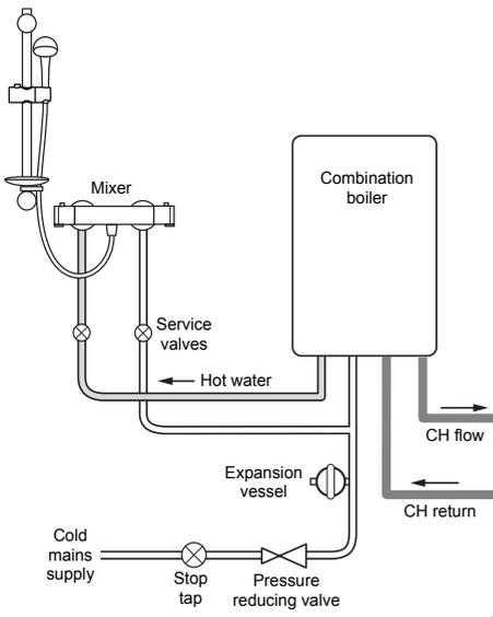
**Fig.3** (diagrammatic view – not to scale)
