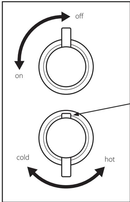
Moving the top lever controls the flow of water, turning anti-clockwise to increase the flow.
