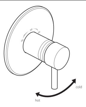
Moving the contol lever anti-clockwise will decrease the water temperature. Pull the handle out to increase the flow of water.
